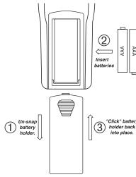
Figure 4. Battery Installation for the VS715's Remote Control.
